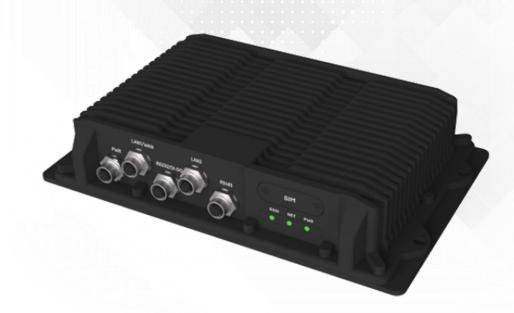
Certified for rolling stock applications, **MegaMesh Rail** is the ultimate broadband connectivity solution for high-speed vehicles and trains. Powered by our patent HyMesh technology, **MegaMesh Rail** combines 5G/LTE capabilities with WiMesh (Wi-Fi6 based) to offer higher data transmission speed for video and other bandwidth-intensive applications.
